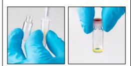
Note: Free dye should not flow through the column and should remain in the upper part of the column. The separation of the free dye is most effective if the reaction volume is between 50-100  $\mu$ L.
